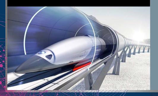
The brainchild of Elon Musk, Hyperloop is a high-speed travel system conducted through low-pressure tubes. The transport pods' projected speeds are inconceivably fast, with engineers aiming for Hyperloop to reach speeds of 600 mph. One Hyperloop project is to create a system that would transport passengers from LA to San Francisco in 45 minutes.
